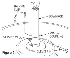
☐ 10. Tighten the setscrews (Figure 6) securely while pulling up on the downrod.
